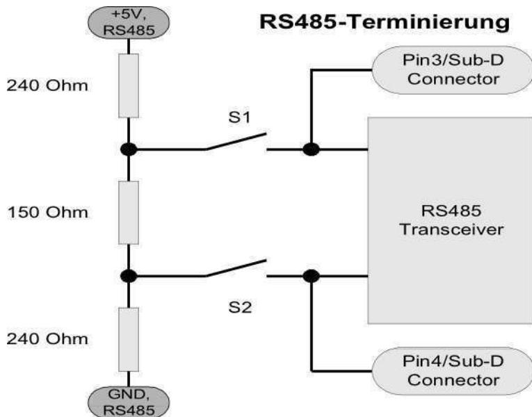
The resulting terminating resistor is approx. 115 ohm.
