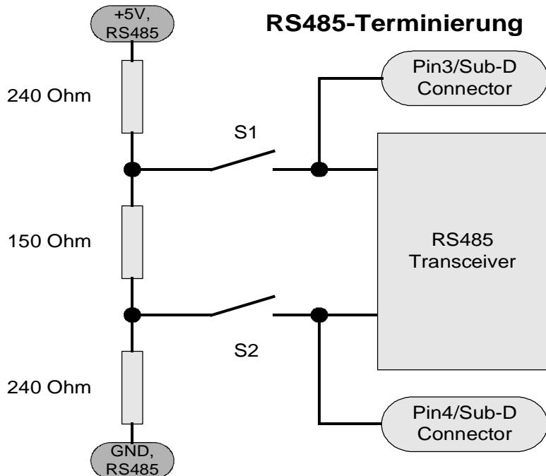
The resulting terminating resistor is approx. 114 ohm.
